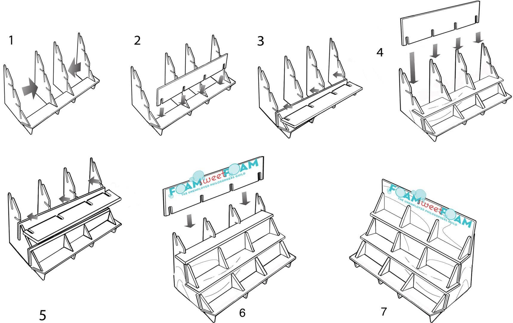
Natural materials, like the wood we use, are prone to irregularities. In some places you will find an area that has been patched or has a small chip. The display is constructed so that the parts can be flipped around, making it possible to construct the display without visible irregularities.
