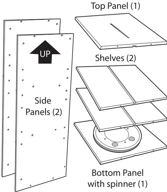
**1.** Carefully unpack and locate all parts before beginning assembly. Use the illustration at left to identify and orient parts.
