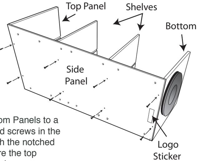
**2.** Attach the Top and Bottom Panels to a side panel with the 5/8" wood screws in the pre-drilled holes. Then attach the notched shelves as shown. Make sure the top panel has the groove facing down.
