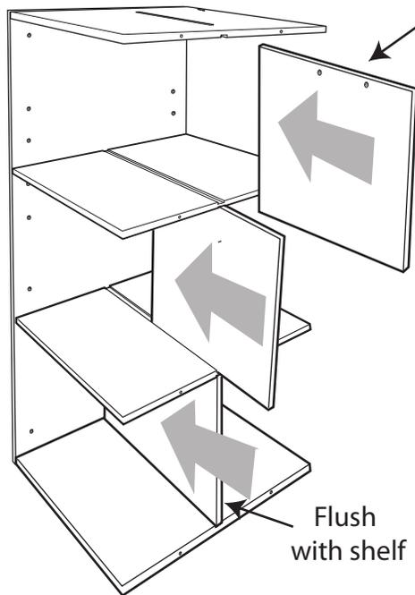
**3.** Slide the 3 dividers into the grooves between each shelf. The divider with the drilled holes goes on the top shelf with the holes at the top. All dividers should fit flush with the ends of the shelves.
